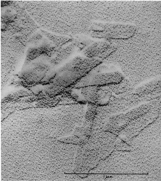
Fig. 2. Scanning electron micrograph of hectorite lamellae. (Reproduced with permission from ICI Plc.)
